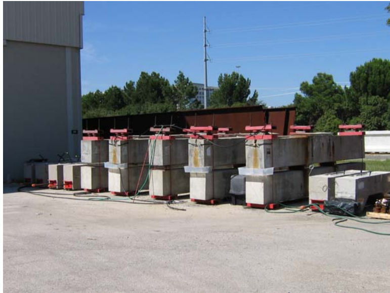
Figure 3.1: Phase II Beams Under Exposure Testing
