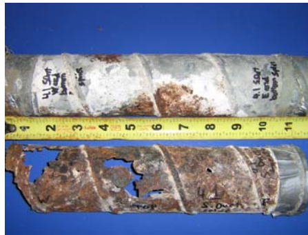
Figure 5.59: Beam 4.1 South Duct Industry Standard Splice
