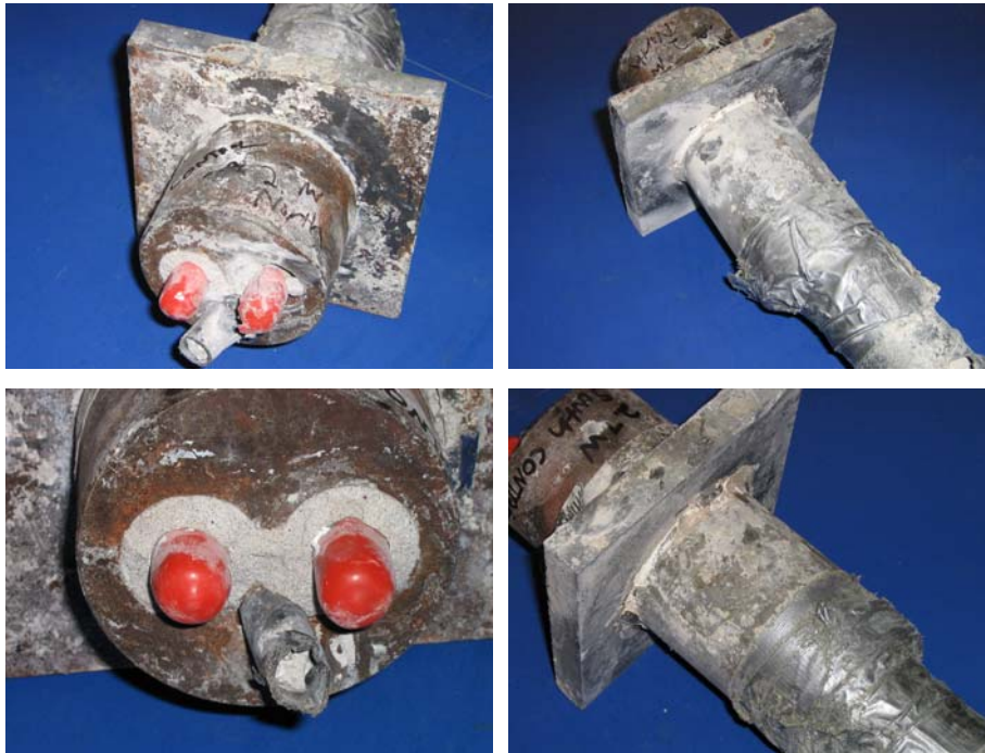
Figure 5.72: Beam 2.7 West End Anchorages After Removal (Controls): North Duct Anchorage (Top, Left and Right), and South Duct Anchorage (Bottom, Left and Right)
