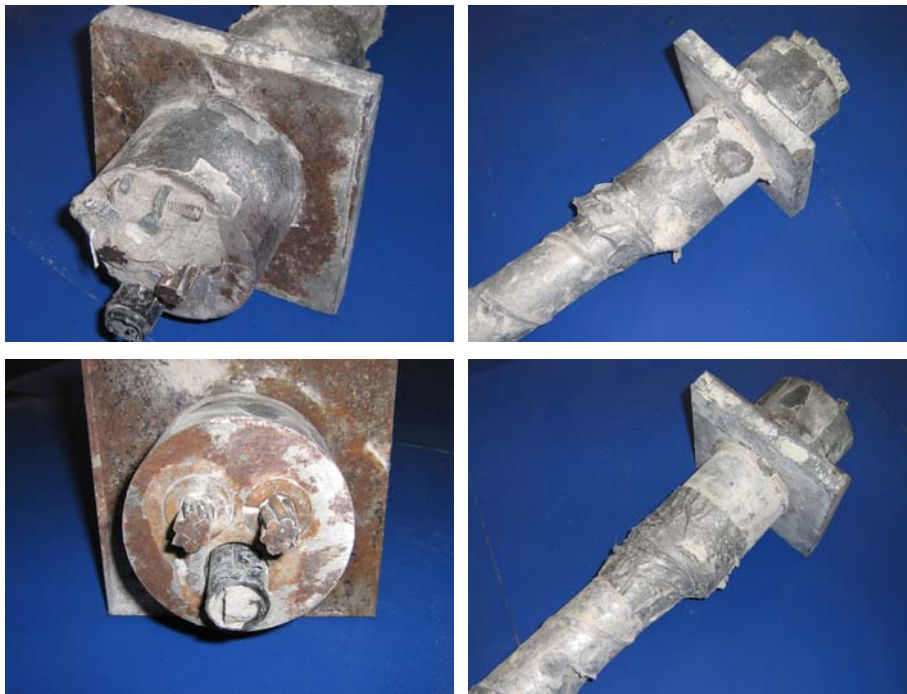
Figure 5.92: Beam 2.9 East End Anchorages (Dripped End)-North Duct Anchorage (Top, Left and Right), and South Duct Anchorage (Bottom, Left and Right)
