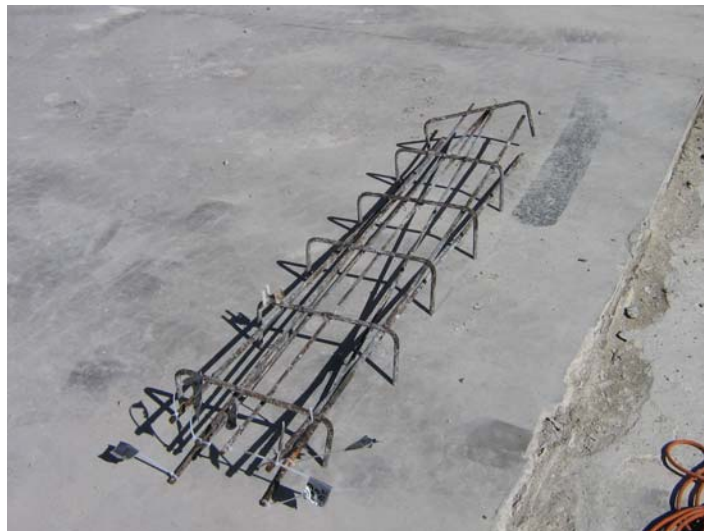
Figure 5.11: Mild Steel Reinforcing Cage After Removal From Beam (Phase II Beam 2.10 Pictured)
