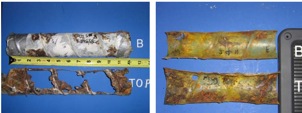
Figure 5.40: Beam 2.4 Duct Splices-South Duct Industry Standard Splice (Left) and North Duct Heat Shrink Splice (Right)
