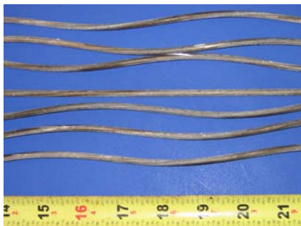
South Duct Strand
