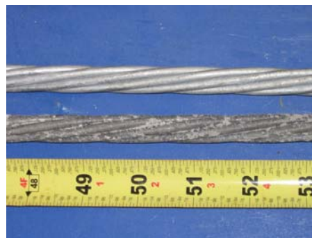
Figure 5.80: Autopsied Galvanized Strand (Bottom) vs. New Galvanized Strand (Top)
