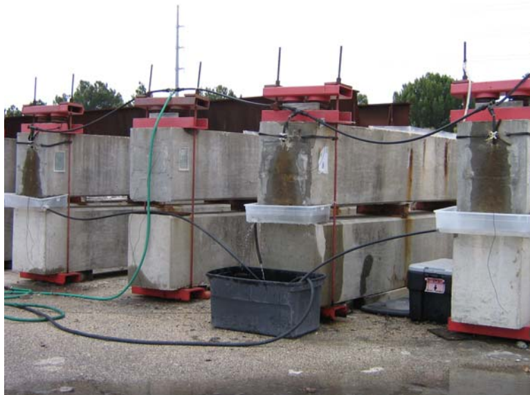
Figure 3.2: Anchorage Exposure System
