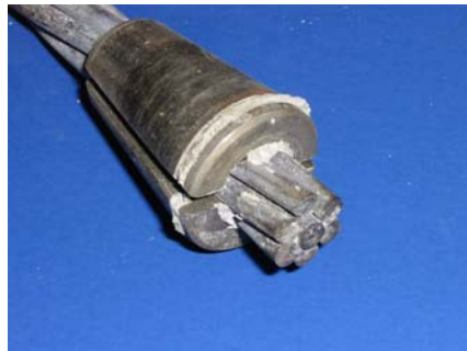
North Duct Strand with Wedges
