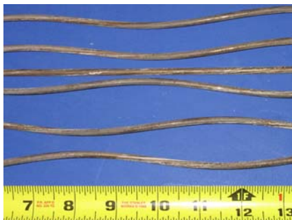
South Duct Strand
