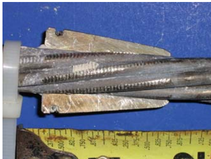
South Duct Strand With Wedges
