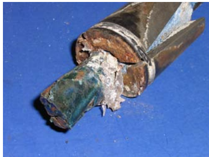
South Duct Strand With Wedges
