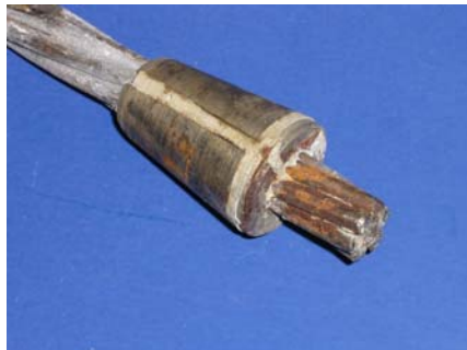
South Duct Strand With Wedges
