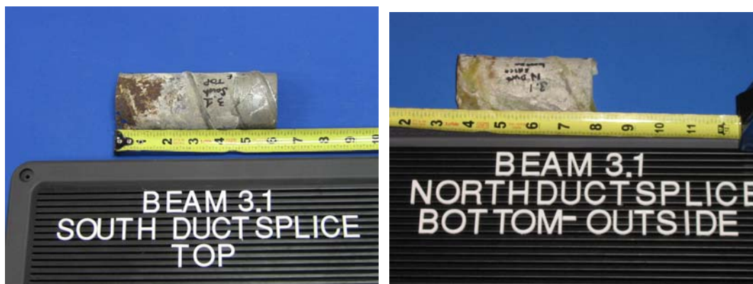
Figure 5.44: Beam 3.1 Duct Splices-South Duct Industry Standard Splice (Left) and North Duct Heat Shrink Splice (Right)
