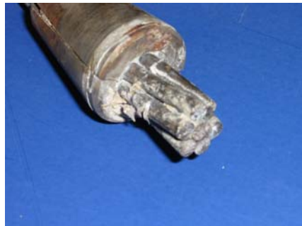
North Duct Strand With Wedges
