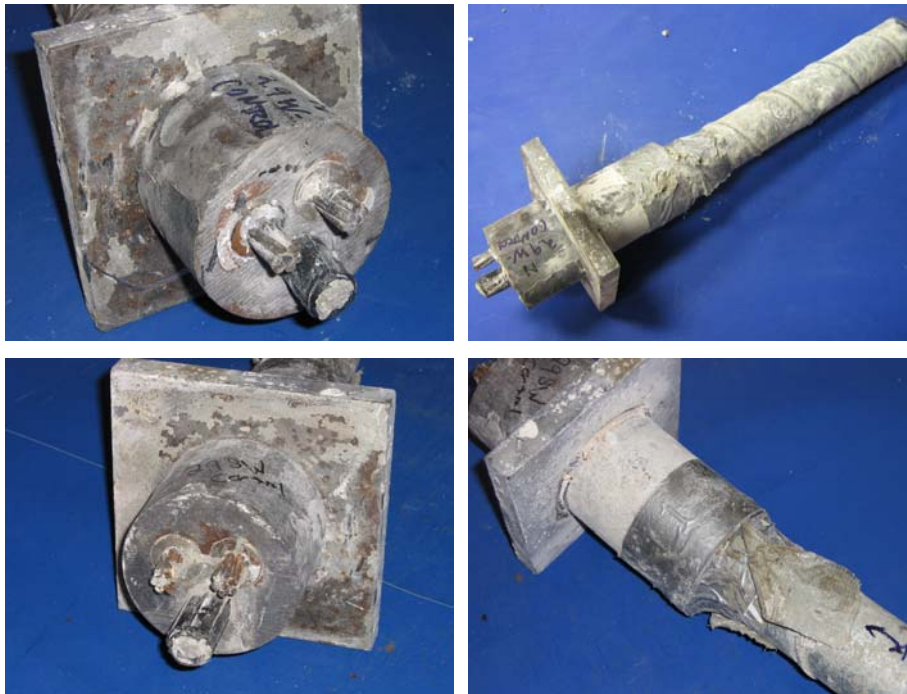
Figure 5.90: Beam 2.9 West End Anchorages (Controls) After Removal-North Duct Anchorage (Top, Left and Right), and South Duct Anchorage (Bottom, Left and Right)
