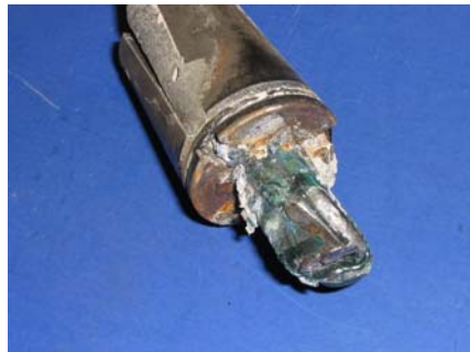
North Duct Strand With Wedges
