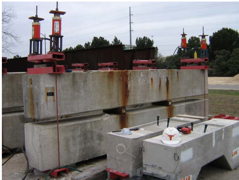
Figure 5.1: Beam Unloading (Phase II Beam 2.9 Pictured)
