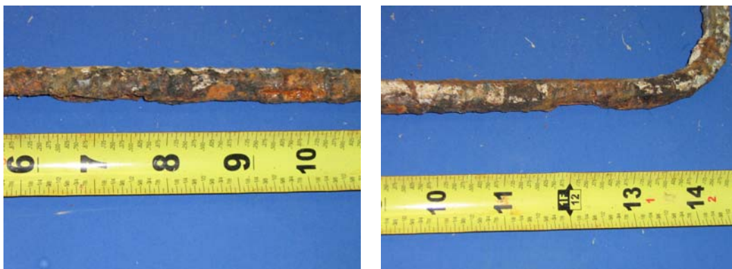
Figure 5.26: Beam 1.4 Autopsy Elements-Longitudinal Bar (Left) and Stirrup (Right)
