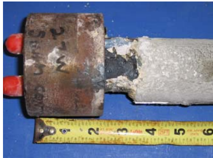
South Duct Grout
